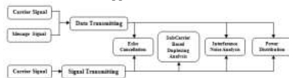
Fig:2 Echo Cancellation Using Duplexing in MIMO OFDM
